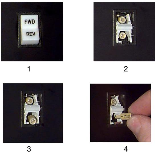
**Figure 3.3 LED Disassembly/Assembly**
