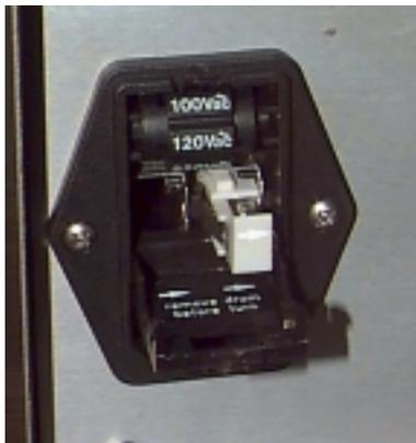
**Figure 3.4 Power Entry Module**
