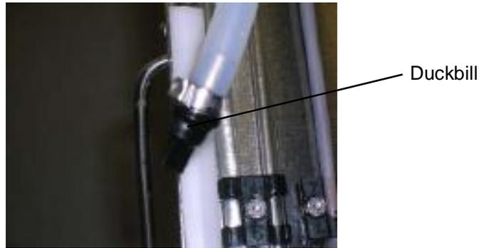
4. With the new bottle right side up, remove the bottle cap and seal and insert the vent tube into the bottle.
