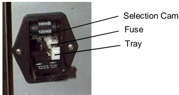
**Figure 2.3 Power Entry Module**
