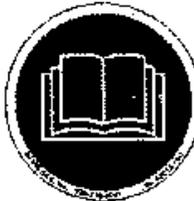
Indicates the operating and Maintenance manual must be read before operating the equipment.
