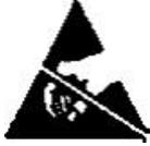
Indicates an electrostatic sensitive component.
