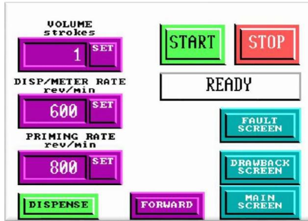
The Volume and Rate screen is used to set volume and rate parameters (See below for a description of each section)
