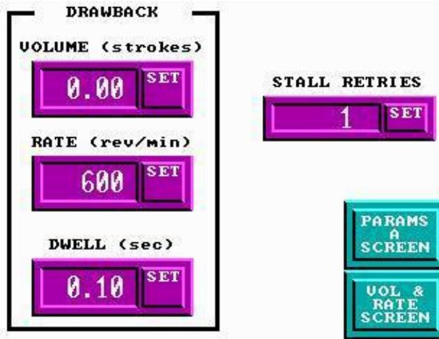
The Drawback screen is used to set drawback and configuration parameters (See below for a description of each section)
