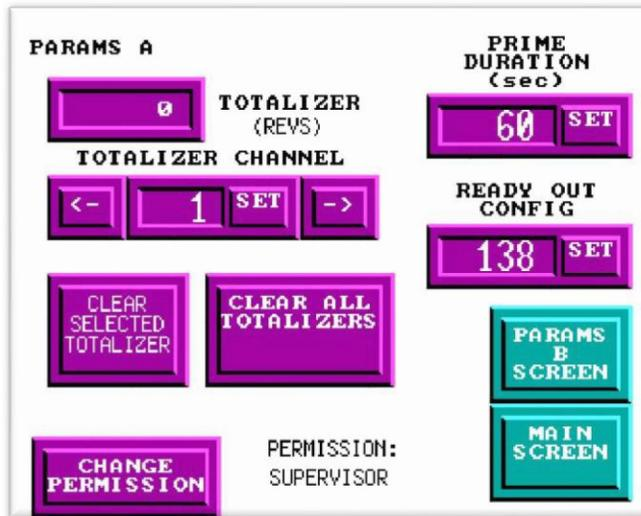
The Params A screen displays system parameters and user information (See below for a description of each section)
